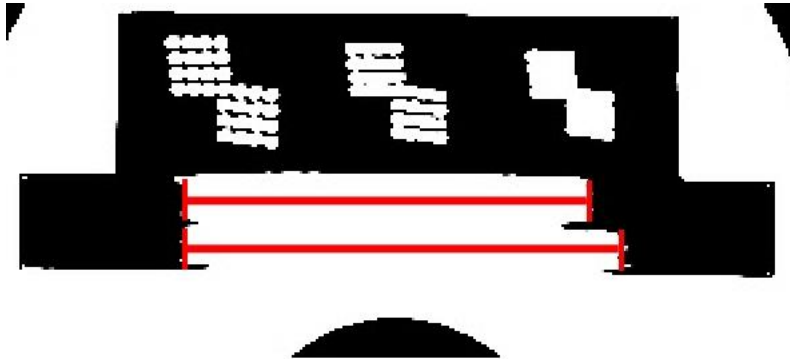
Figure 12. Magnified region of slice 1 showing signal ramps with display window at zero and the level at half the average signal level of the ramps. The length measurements for the ramps are shown on the image (lines).
