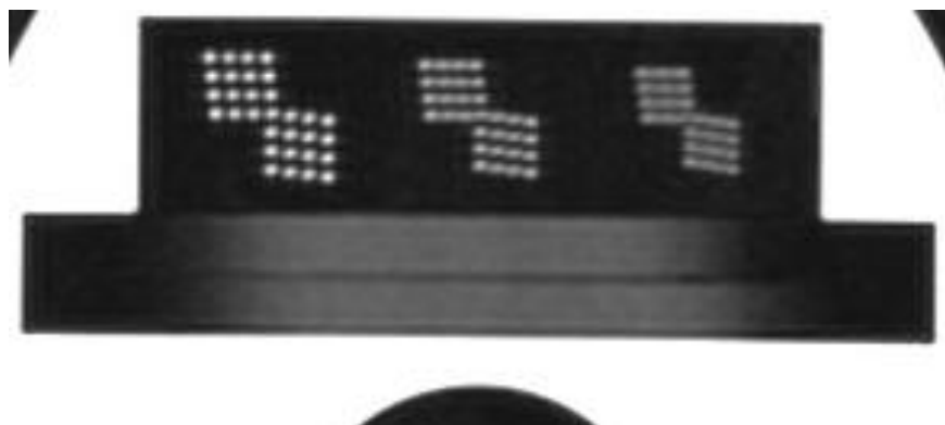
Figure 8. Magnified portion of slice 1 displayed appropriately for visually assessing high contrast resolution.
